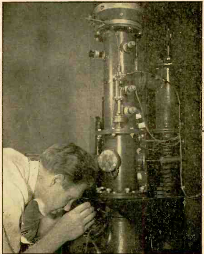
Dr. Gulbransen inspects the target of his "machine-gun." This three feet of steel pipe is a genuine electron tube, in spite of the fact that it resembles a section of water main more closely than it does one of the tubes in your radio. The associated apparatus is used to maintain the vacuum and control the admixture of traces of desired gases, when required.
